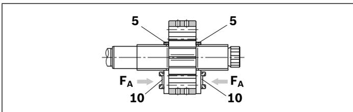
The axial compensation force  $F_A$  acts in the area of the pressure chamber and is generated by the pressure zone (10) in the axial discs (5).
