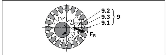
The radial compensation force  $F_R$  acts on the segment (9.1) and segment carrier (9.2).
