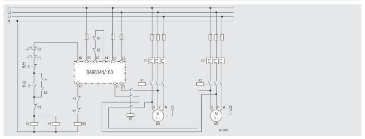
BA 9034N/100 simultaneous braking of 2 motors in serial connection
