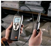
testo 625 with probe head attached by cable
