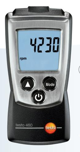
The especially handy, pocket-sized rpm measuring instrument testo 460 optically measures rpm, e.g. on ventilators and shafts. The ideal distance to the measurement object is between 10 and 40 cm. Simply attach a reflective marker (optional) to the measurement object, point the visible measurement spot at the reflective marker, and measure. Min./max. values are directly displayed at the press of a button.
